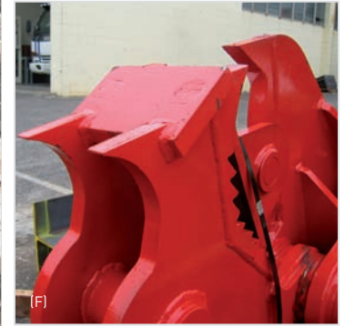
IMAGES: (D) & (D Insert) Down sizing timber; (E) Wood Shear profile; (F) Showing the new stump ripper claws on the lower jaw
