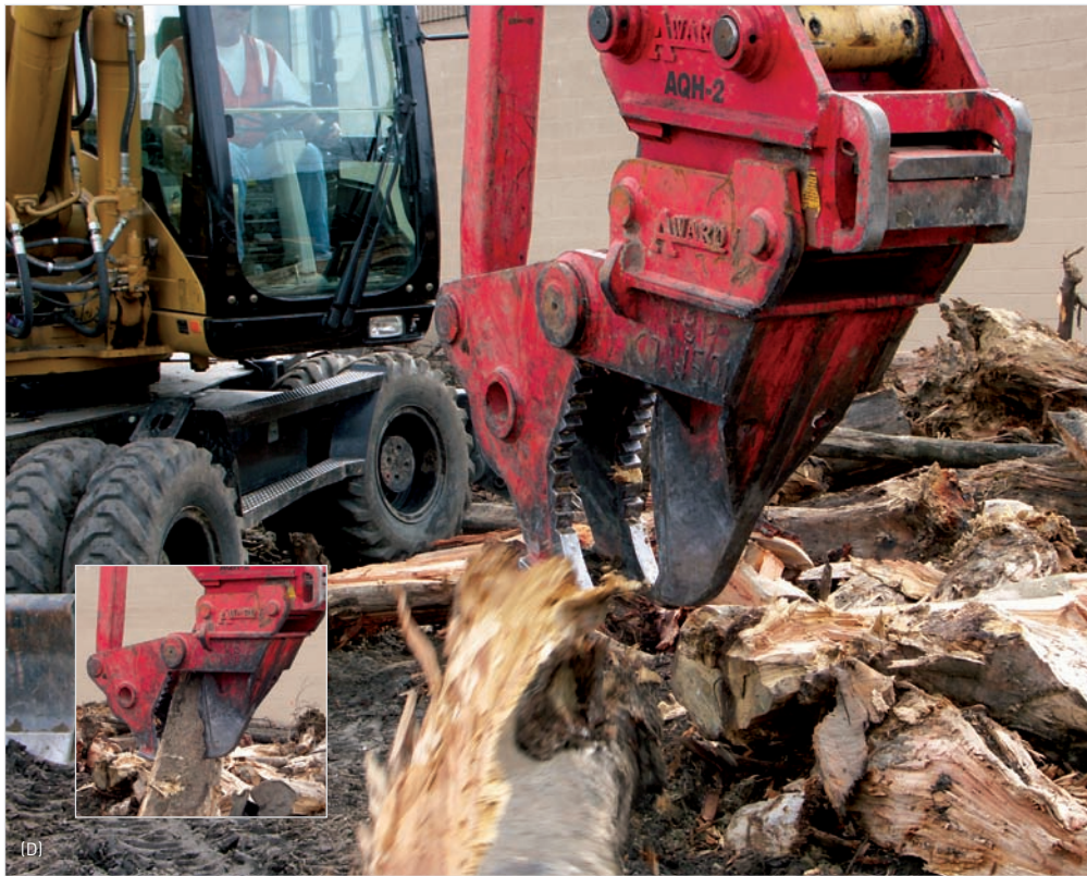
IMAGES: (D) & (D Insert) Down sizing timber; (E) Wood Shear profile; (F) Showing the new stump ripper claws on the lower jaw
