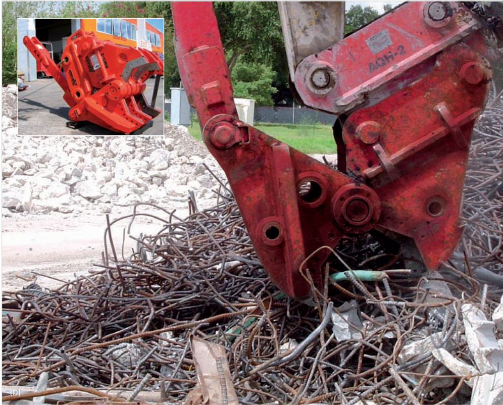
IMAGES: (D) & (E) Re-bar Shear in action; (D Insert) Showing structural fabrication strength; (F) Added value cut Re-bar product
